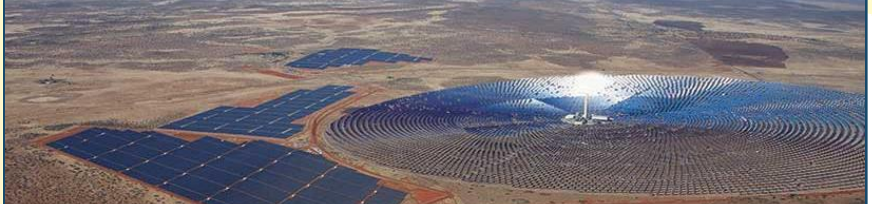
Integration of PV and CSP near Postmasburg, South Africa [5, 6]
