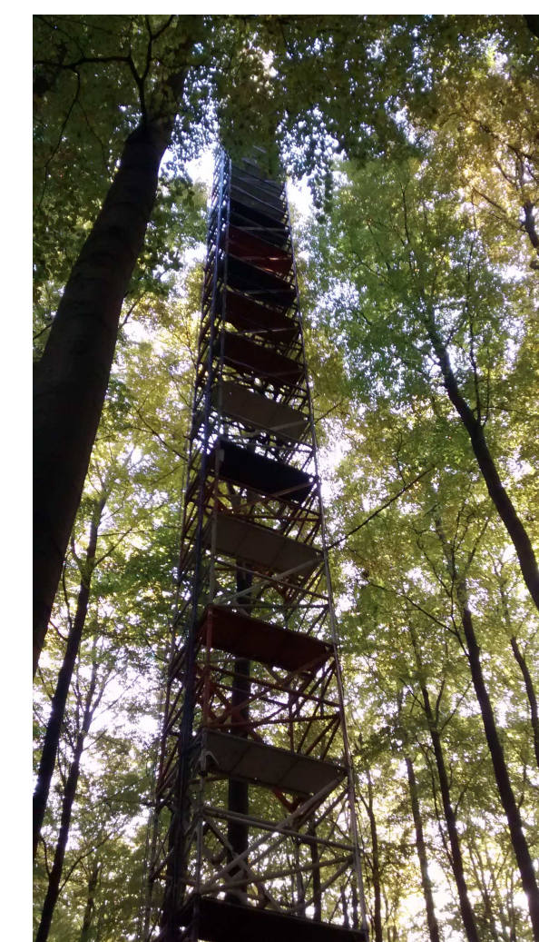
Figure 1: Field site: Eddy Covariance tower in a managed beech forest in Germany
